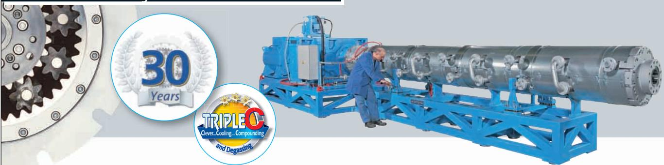
**The ENTEX Planetary Roller Extruder - The most powerful extrusion system for your demanding tasks.**
