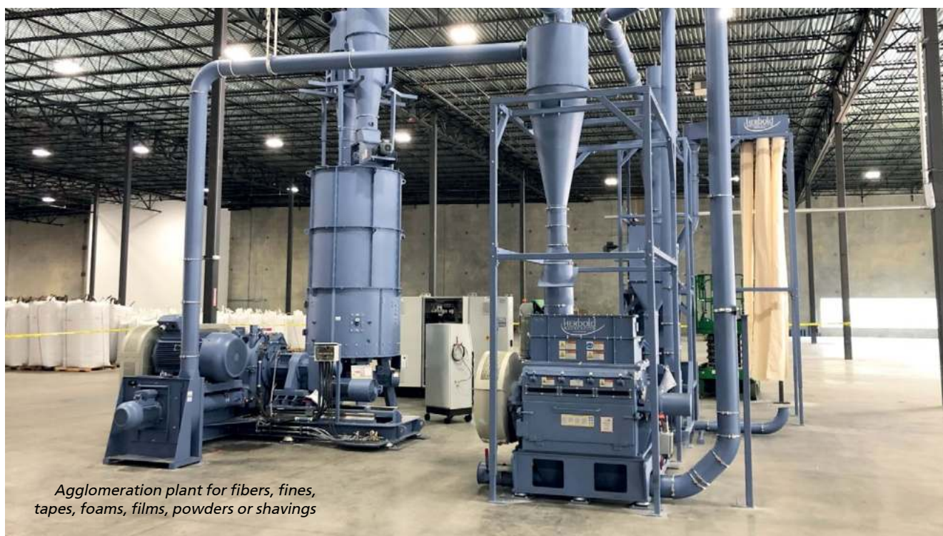
The HV 70 Plastcompactor is the most powerful of the series from Herbold Meckesheim (All pictures: Herbold Meckesheim)
