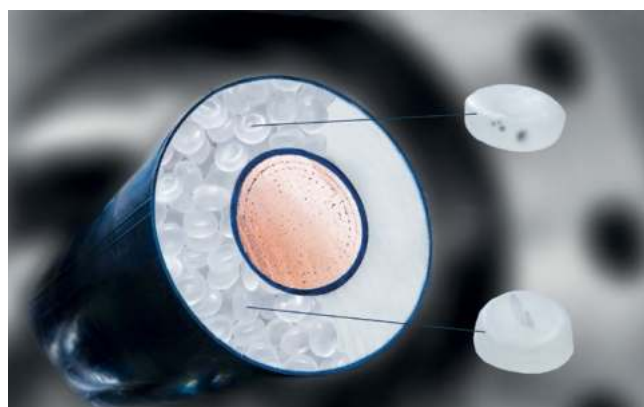
Impurities such as metallic particles can affect both XLPE and PP. The PURITY SCANNER ADVANCED detects the smallest contamination in the material – before they enter the extrusion process
