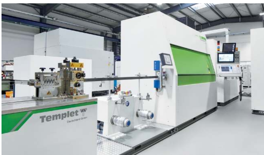
LASER LINE, manufactured by Templet Deutschland GmbH. Sophisticated measuring and automation solutions for efficient high-speed production of aluminium multilayer pipes (Picture: Templet)
