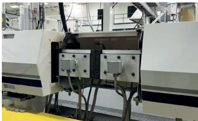
Oven style guards for high heat retention, cast bronze and aluminum heaters use a targeted energy theory to deploy energy where the process demands it
