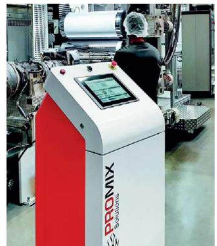
*The inline viscometer "Visco P" measures the actual viscosity under processing conditions and in real time (All images: Promix Solutions AG)*
