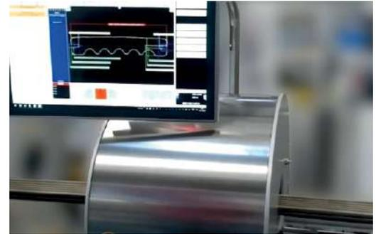
*ProfilControl 7 WPC is the system of choice to ensure perfectly shaped decking and cladding boards made of wood-plastic composites. This system checks the entire contours and surfaces of decking boards in a continuous inline process*
