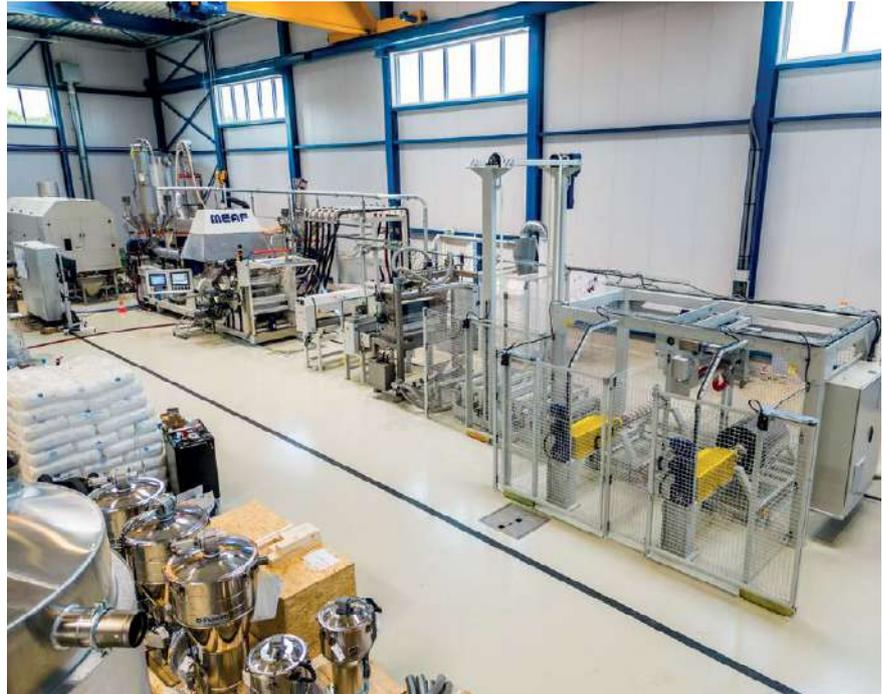
of post-consumer PET flakes for food packaging, combining crystallization and drying in a single process. The system operates without vacuum technology and can be retrofitted on existing extrusion lines. The efficiency of the cleaning process has been verified by a Letter of Non-Objection from the US Food and Drug Administration (FDA), while tests have shown compliance with the European Food Safety Authority (EFSA) criteria for the use of recycled materials for direct food contact packaging.
