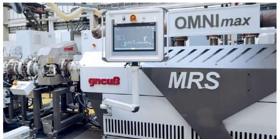
*Gneuss OMNImax Recycling Machine with MRS extruder and RSFgenius filtration system*
