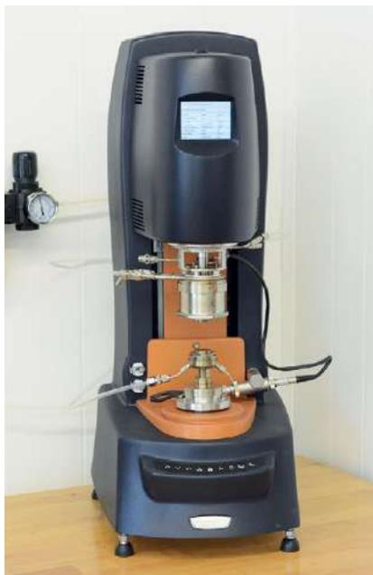
TA Instruments DTC-300 Thermal Conductivity Meter
