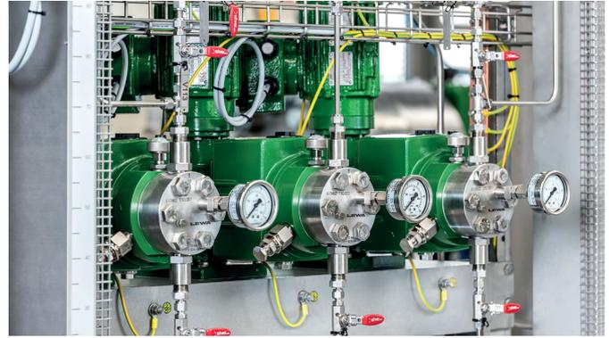
*LEWA Smart Control guarantees metering accuracy. The controller handles this by carrying out a variance analysis and then instantly adjusting the flow rate as necessary (Source: LEWA GmbH)*
