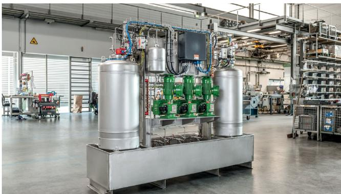
Smart Control" technology and a high precision mass-flow meter. Continuous guide signal and measuring instrument feedback ensure sensitive and prompt control with only very minor deviations. Since the metering systems are being used worldwide, minor modifications were necessary for adapting to national regulations.
