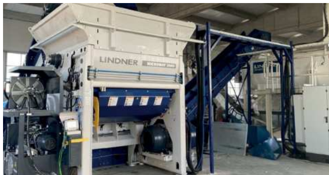
The stationary single-shaft shredder Micromat 2000 reliably shreds the input material, creating the basis for stable downstream recycling processes
