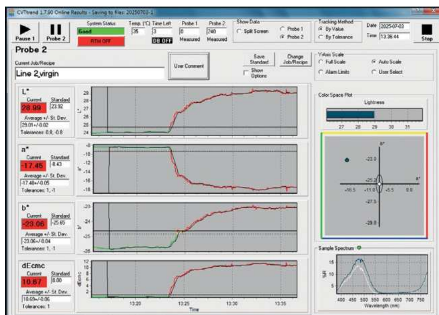
Picture 2: ColVisTec CVTrend Inline Software Showing in Real-Time Variations of Recipe
