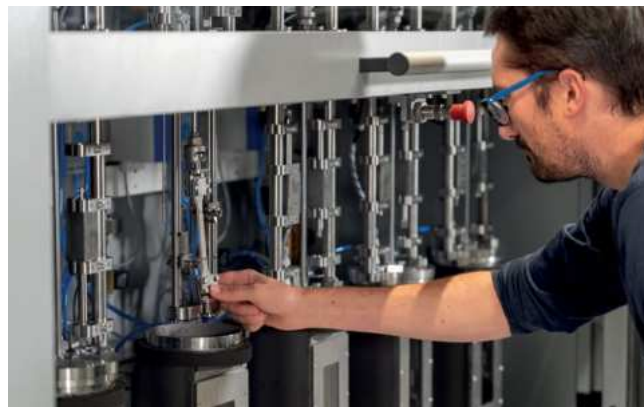
Newly developed testing facility (consisting of six independent measuring stations) for determining the influence of media on the stress crack resistance of plastics (Photo: Luca Hoffmannbeck/SKZ)
