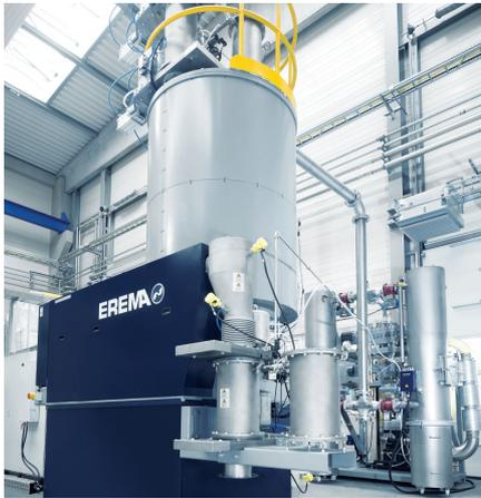
The MPR from EREMA allows the decontamination, drying, dedusting and crystallisation of different PET input materials already prior to extrusion. Photocredit: EREMA, Humer / Wallmen
