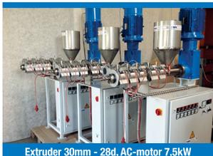
Extruder 30mm - 28d, AC-motor 7,5kW
