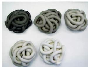
*Application example: Asaclean PF used to clean PEI (black). Injection moulding machine: 50 ton, Barrel temperature: 380°C. Quantity of Asaclean PF used: 500 g*
