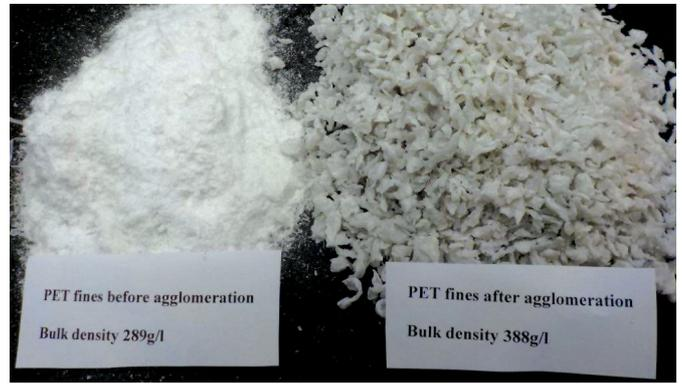
Fig. 3: PET dust before and after compacting in a Herbold Plastcompactor
