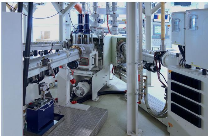
*Fig. 4: The 7 layer foil machine is constructed in three functional levels on top of each other. On the lowest level (not visible here) there are three extruders (see Fig. 3), on level two there are two extruders for the cover layers, on the top level the dosing units to supply the extruders situated below*
