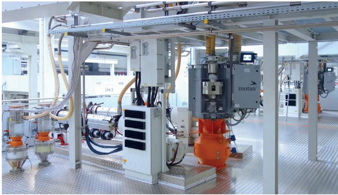
Fig. 5: Central mixing station to supply the "regrind extruder". In this, four material components come together (regrind from the silo or from the BigBag, stabiliser for the adhesion promoter and new PP material) which are added from the gravimetric dosing units on the third level. Photo 2-5: Author
