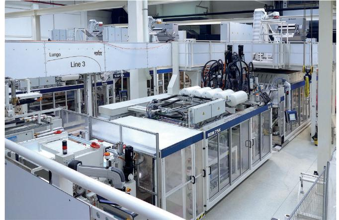
*Fig. 2: The 7 layer barrier foil which comes out of the extrusion machine runs directly into a multi cavity deep drawing and punching machine. The remaining punched frame and any bad parts produced are then fed directly into a cutting mill (in the background at the end of the machine) and fed back into the production line from there*
