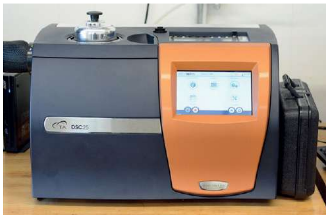
The rheology lab's scanning calorimeter
