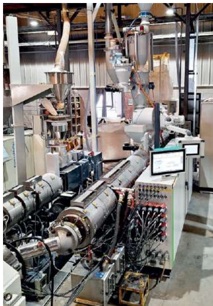
Twin screw extruder twinEX and coextruder conEX with permanently installed gravimetric dosing unit
