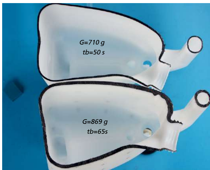
Picture 2: Comparison of the results which have been obtained using a conventional conical die (on the bottom) and those that have been reached using a cylindrical GWDS die (on the top)
