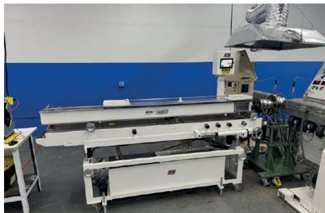
Fluidized bath in the test extrusion facility
