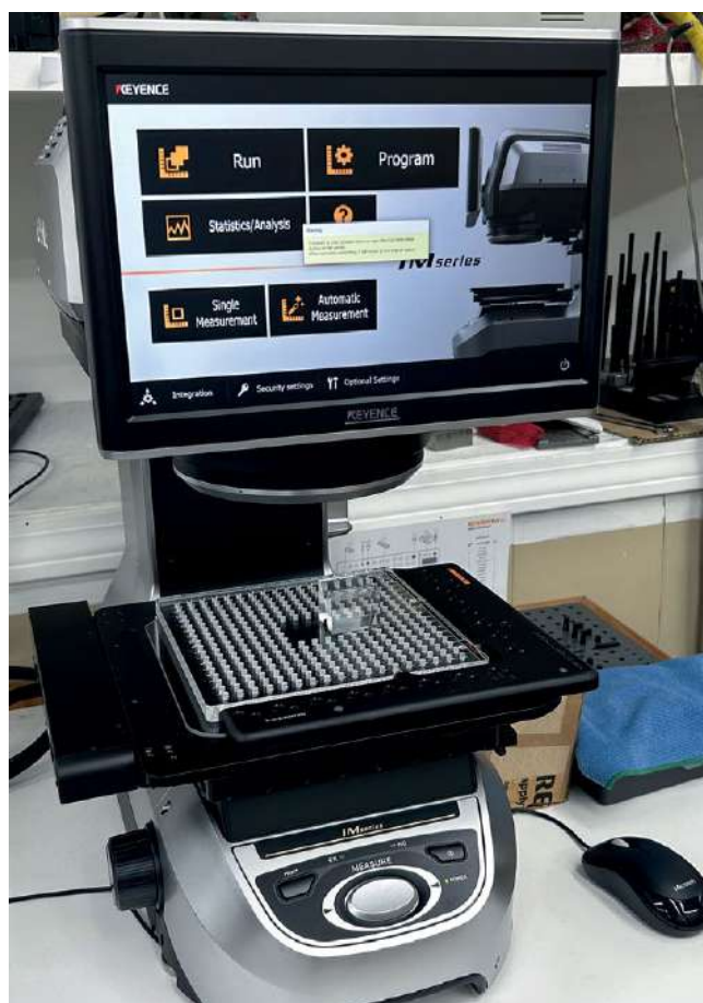
Close-up of the IM-8000 Series, a dimensional measurement system
