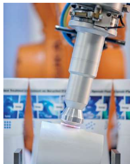
Openair-Plasma treatment of a recycled plastic cup. Plasma pretreatment makes recycled plastics more usable, allowing them to be recycled and reducing waste (Copyright: Plasmatreat GmbH)
