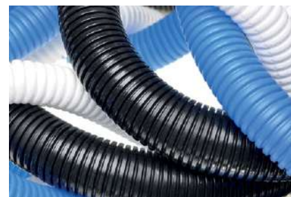
Extruded pipes made of halogen-free flame-retardant polypropylene, which are used, for example, for guiding electrical cables, protecting optical fibres or for supplying and discharging media, prevent the spread of fires (© shutterstock/Flegere)
