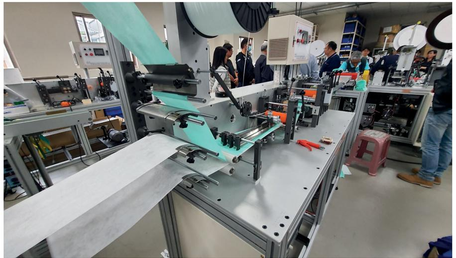
Such capacity expansion was at first estimated to take six months – much too slow compared to the speed at which COVID-19 spreads. But it ended up taking only 40 days to build up all the 92 sets of automated mask production lines with support from the machine tool industry.
