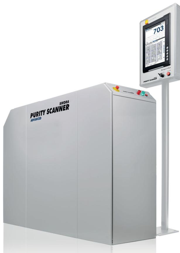
*The online inspection and sorting system detects metallic contamination inside the pellet as well as black specks and burns on the pellet's surface*
