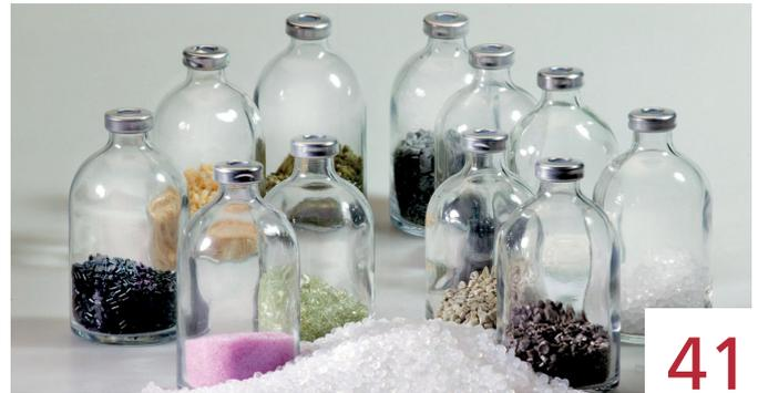
**41** Plastic recyclates often have off-odors, some of which have not hitherto been identified. The Fraunhofer Institute for Process Engineering and Packaging IVV (Germany) has analyzed the sensory properties of post-consumer shopping bags made of low density polyethylene (LDPE) and originating from different collection systems.
