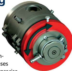
Features of the single-point crosshead include a patented cam-lock deflector for quick changeovers, with a residence time of one minute at .5 lb/hr material flow, optimized usage with extruders measuring 1/2" and 3/4", and a max die ID of .250."
