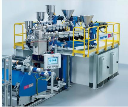
*BREYER TubeFlex multilayer flat film extrusion*
