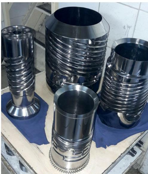
The adapterblock works like a feedblock bringing the melt A from extruder A to the inner or middle or outer layer depending on the product.
