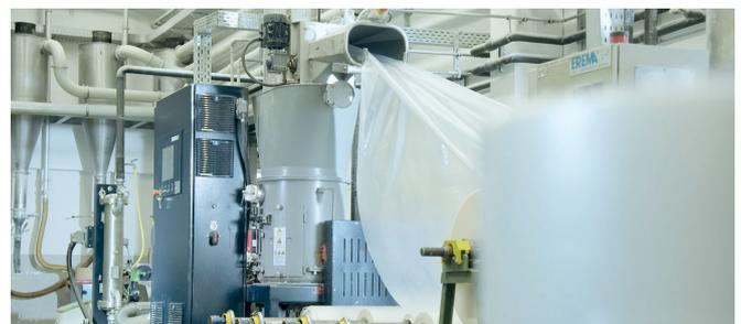
EREMA offers a fully automatic processing system for edge trim with the proven INTAREMA® K. Sales have increased by 100 per cent compared to the previous financial year. More and more producers are reducing their material costs by recycling clean production waste.
