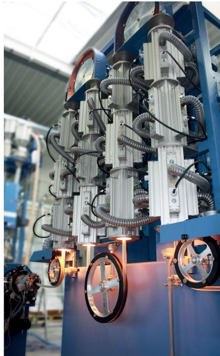
*Picture 2: PEXLINK conveyor oven – Infrared units are the prerequisite for the optimum cross-linking of polyethylene. To protect the pipe from burining, a cooling system is part of the oven*
