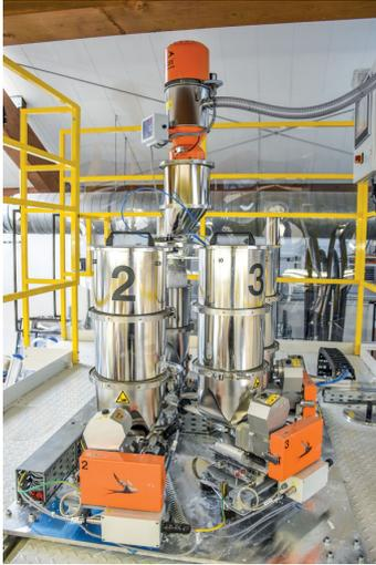
*Pic. 3: The dosing system is controlled by a Gravinet GP control unit, which is operated using a menu displayed on a 12.1" TFT touch screen*
