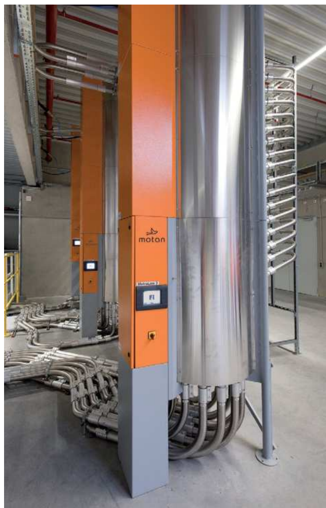
Fully automatic Metrolink coupling station (Source: motan)
