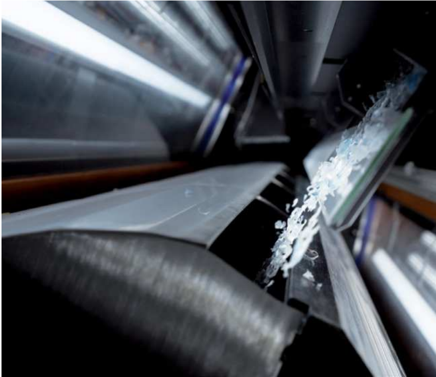
INNO-SORT™ FLAKE detects flakes by polymer type, color and transparency in a single sorting step, ensuring precise separation even at small particle sizes
