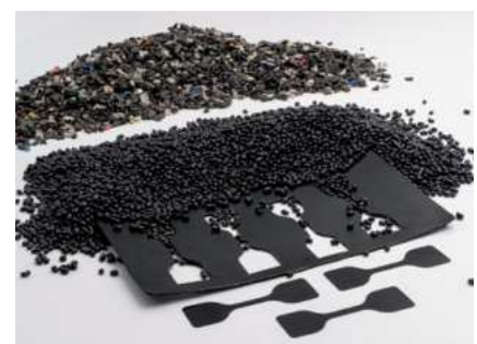
Milled material, recycled compound, film, and test specimens for the strain hardening test (Photo: Luca Hoffmannbeck, SKZ)
