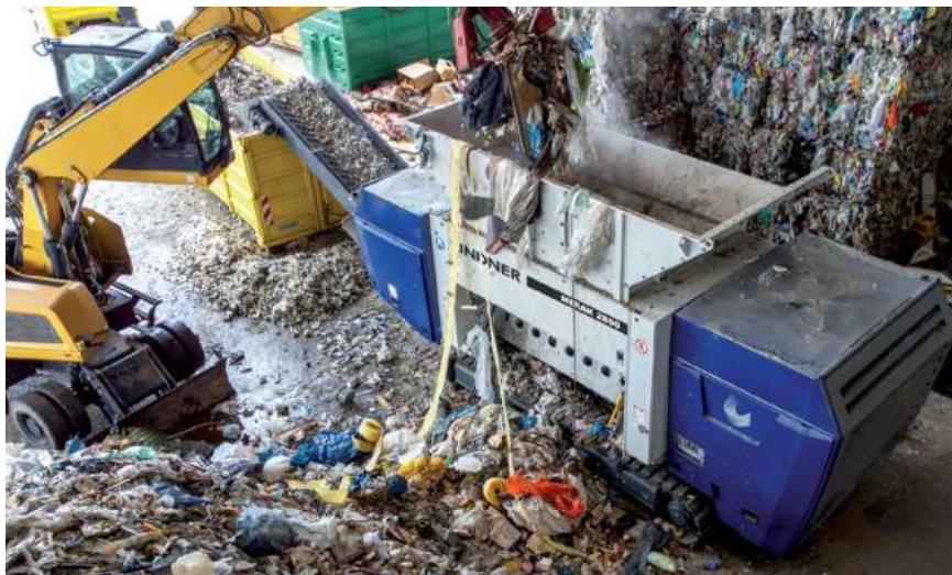
The Merak 2800 is a powerful universal shredder for the most diverse materials and – depending on the application and screen configuration – makes it possible to produce defined output sizes from 30 to 120 mm. At IFAT, Lindner will be presenting the established shredder with its new drive concept that significantly expands the range of application (Picture: Lindner)
