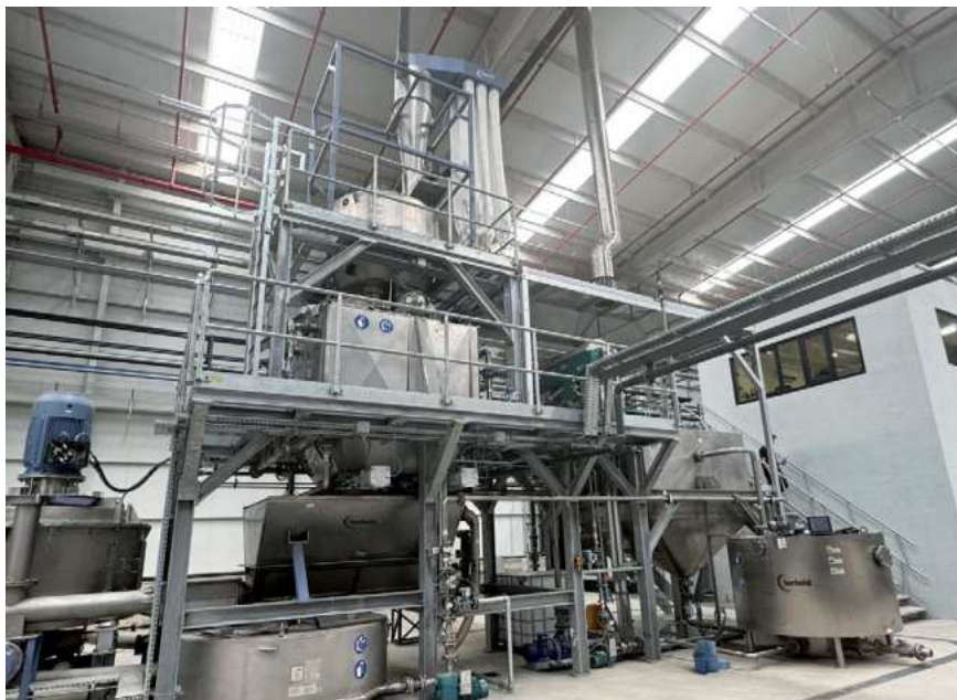
The two SMS forced feeding granulators installed in the first line ensure uniform flake size and stable material intake, creating ideal conditions for downstream washing and density separation processes (Photos: Herbold Meckesheim, Germany)
