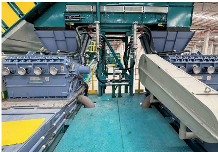
As a central process stage within the PET washing line, the hot wash system in batch design enables controlled temperature management and defined dwell times for efficient removal of labels, adhesives and organic residues
