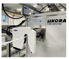
HÖHLE uses the X-RAY 6000 PRO for dimension measurement during the production of microducts
