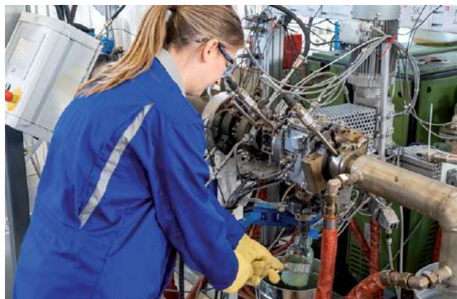
Sampling of reaction products from the continuous chemical recycling process (Photo: Luca Hoffmannbeck, SKZ)
