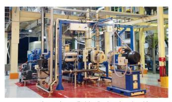
New polypropylene pelletizing line in Indonesia, with Useon's SAT-X 175 co-rotating twin-screw extruder; skid-mounted BKG® underwater pelletizer is in foreground
