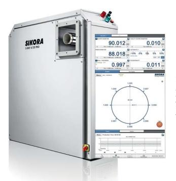
The X-RAY 6000 PRO is used, amongst others, for wall thickness measurement of light metal alloy tubes as well as the layer thickness of the plastic coating on steel tubes
