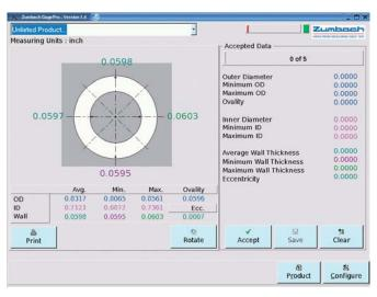
ness, inside diameter and outside diameter are measured instantly. In addition, the ovality and eccentricity can be determined.
