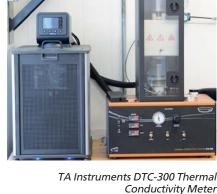
TA Instruments DTC-300 Thermal Conductivity Meter
