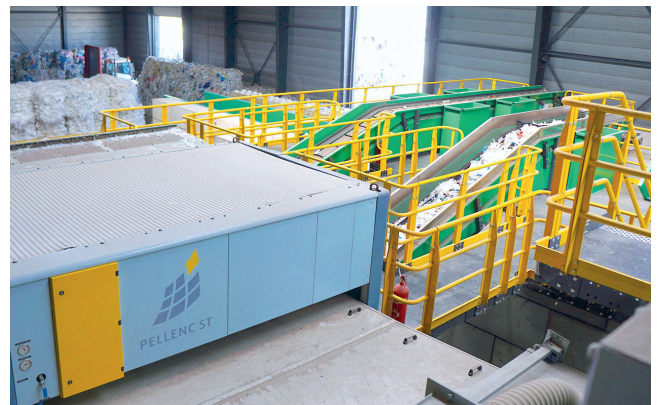
Image 3: The film bales are dissolved at DALY Plastics. They then go through a sorting process that eliminates foreign material and separates the films into color classes or material quality. This is used to produce unmixed bales, which are processed into granules in the recycle plant
