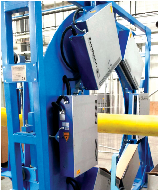
3-axis ODAC 550 system, measuring an Offshore cable of 500 mm OD
