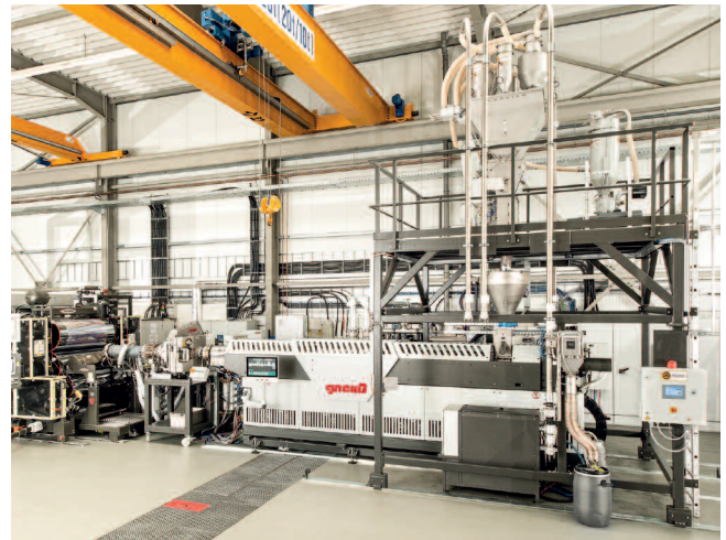
片材生产线含MRS多螺杆挤出机，RSFgenius旋转过滤系统和VIS在线粘度测试仪和PET发泡模型 Sheet extrusion line with Multi Rotation Extruder MRS, Rotary Filtration System RSFgenius, Online Viscometer VIS and PET foam module
