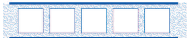
Picture 2: Three-layer micro-foaming hollow board made from GMA new patent hollow die
