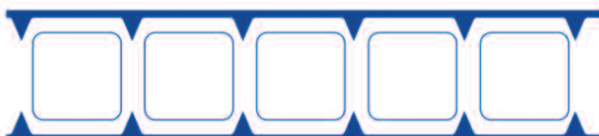
Picture 1: Traditional hollow die design is easy to get problem on surface indentation
