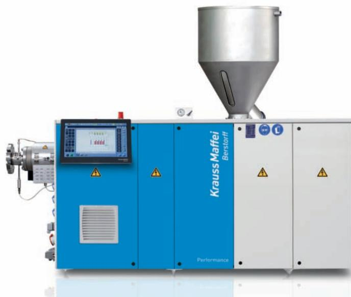
*The KMD 63 KIR conical twin-screw extruder from the Performance series – introduced to the market at the Chinaplas show for the first time*
