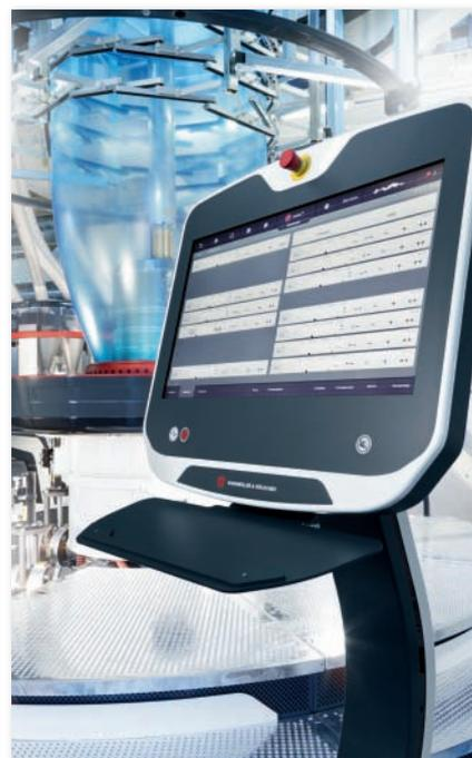
on of a particularly thin breathable diaper back sheet film of only 12 g/m<sup>2</sup> – a product that is predominantly produced in cast film extrusion and with a higher basis weight. Andreas Hoppe, customer service consultant for extrusion systems is convinced that "There is a clear trend toward blown film. Blown films will re-
