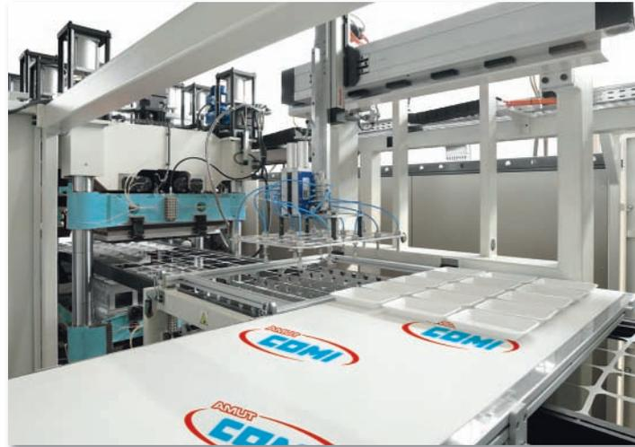
with a T-IML system (In-Mould Labelling for the thermoforming sector), based on a side entry robot to load labels inside the forming mould in order to decorate the articles.
