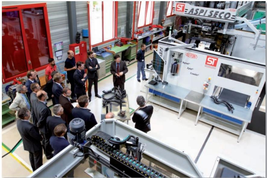
companies. The delivered blow moulding machine model ST ASPI SECO is suitable for the production of parts with materials in monolayer, coextrusion or SeCo (Sequential Coextrusion), in case of need to produce items requiring different mechanical or chemical properties in predefined areas, usually for the automotive industry.
