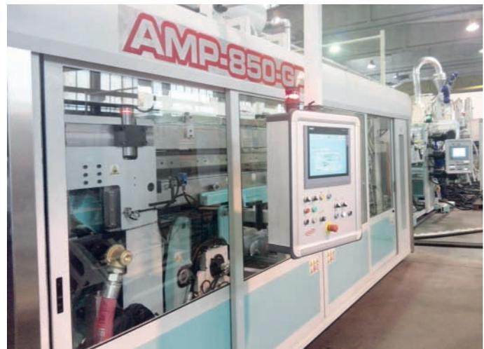
ing is around 700 kN. The output is 115.500 cups/hour with 35 cycles per minute.
