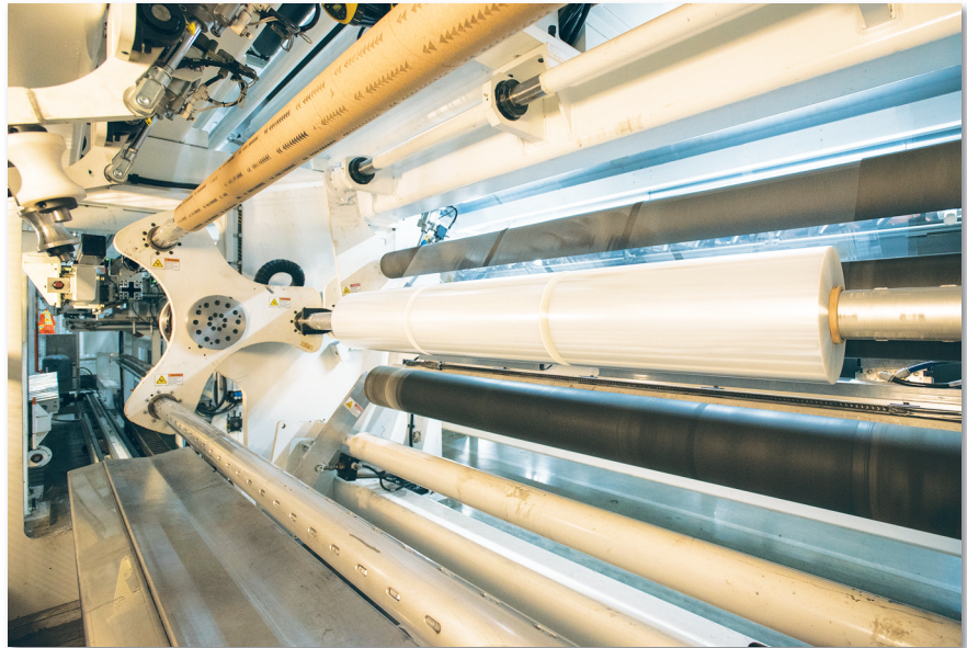
Pictured is Davis-Standard's S3 winder, which enables maximum slit widths for hand-wrap, machine-wrap and jumbo rolls to support multiple market segments
