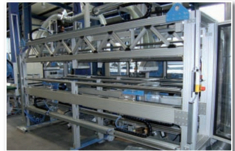
Slitting RB 2 with four sawing stations
