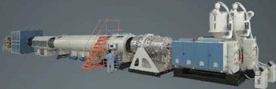
**Large Diameter HDPE Water Supply And Gas Supply Pipe Extrusion Line**
