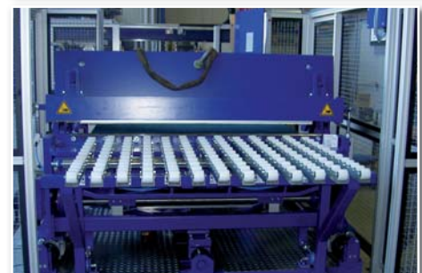
Transverse separating cutter QSS, inlet
