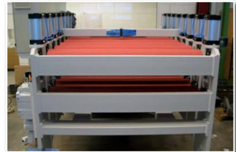
Roller withdrawal AZ 8, outlet side
