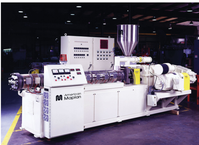
Extrusion machinery from the year 1999: TS-88 extruder for profile extrusion
