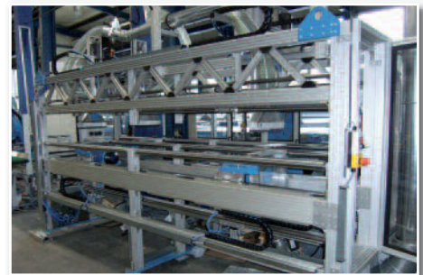
Slitting RB 2 with four sawing stations
