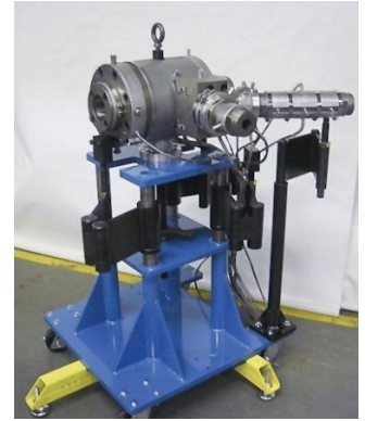
Fig. 2: Extrusion tools require a disassembly/reassembly cart as shown here. This allows precise realignment and prevents costly collisions that damage the die sections and product integrity
