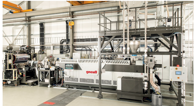
Sheet extrusion line with Multi Rotation Extruder MRS, Rotary Filtration System RSFgenius, Online Viscometer VIS and PET foam module
