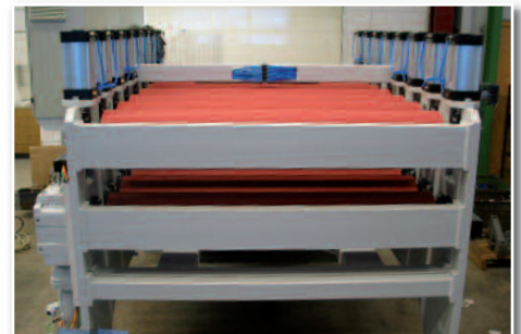
Roller withdrawal AZ 8, outlet side
