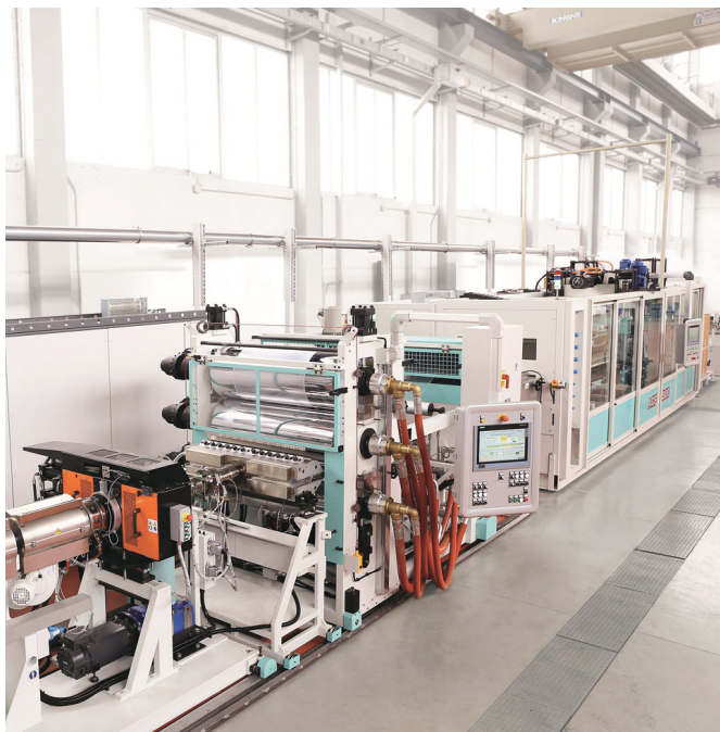
In line thermoforming plant
