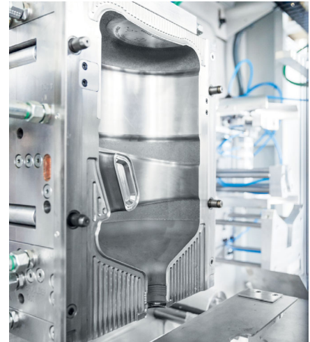
View into the open blow mould with multi-zone temperature control for the production of a water bottle container made of PC
