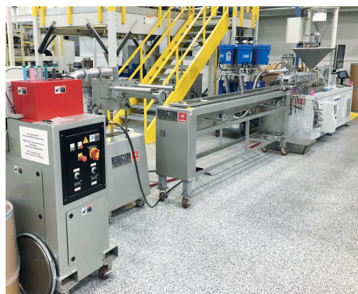
ZE 28 BluePower laboratory extruder produces color masterbatches economical and in high quality
