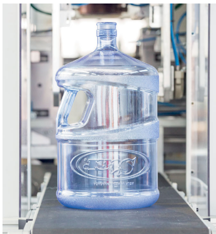
Highly transparent PC container with handle on conveyor belt for directional article output
