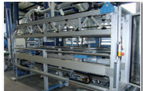
Slitting RB 2 with four sawing stations
