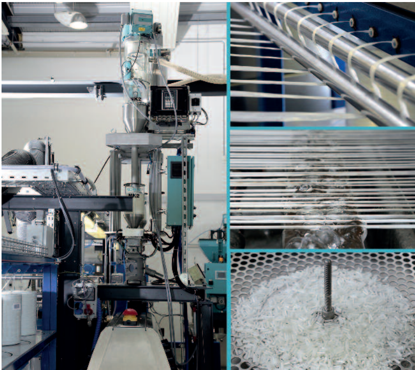
ProTec's LFT pultrusion technology produces high grade long-fibre-reinforced pellets with a wide range of polymer matrices and huge variety of reinforcing fibres. This technology also permits reliable and flexible adjustment of matrix properties (Photo: ProTec Polymer Processing)
