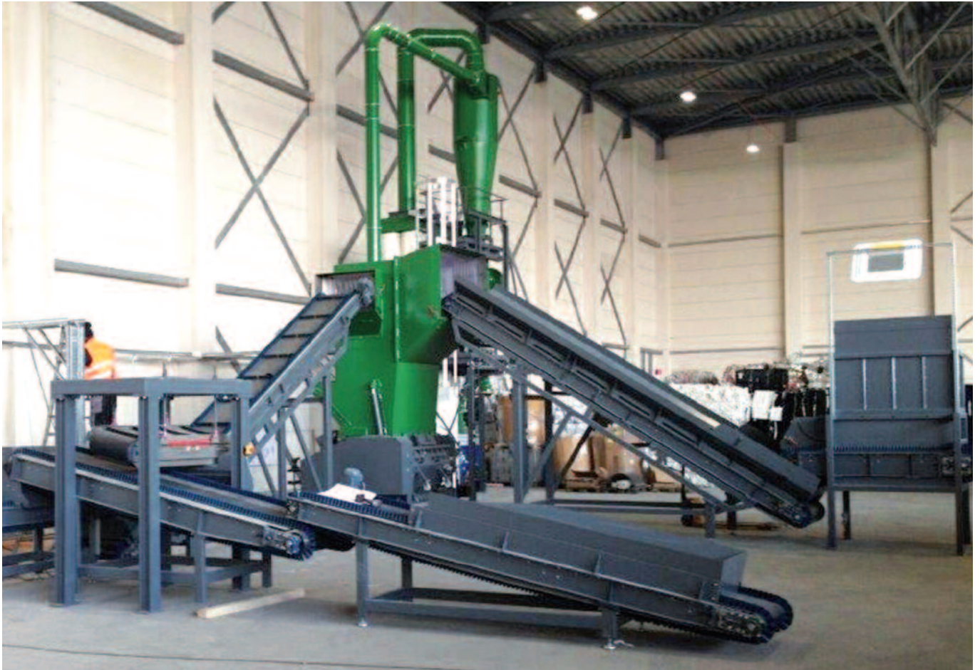
Total granulating solution from Getecha: The large Rotary Cutter granulator RS 6015 (green) with conveying periphery (grey) and cyclone separator (green)
