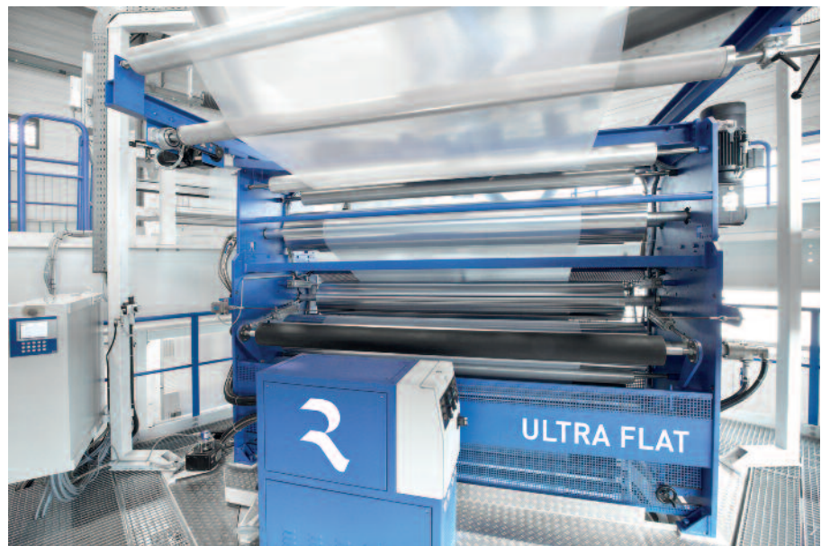
EVOLUTION Ultra Flat take-off system optimizes the film flatness in blown film lines
