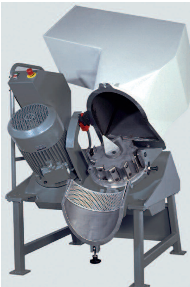
Powerful work horse: The large grinding chamber and the oblique rotor of the GRS 300 granulator allow granulating bulky sprues from injection moulding
