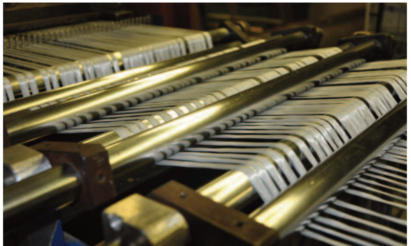
Roving pre-warming with spreading of the individual fibers enables the best individual fiber wetting (Photo: ProTec Polymer Processing)
