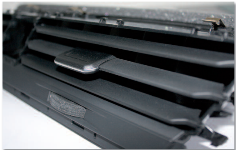
Low moisture absorption results in good dimensional stability, thereby ensuring consistent operating forces during adjustment of the longer slats
