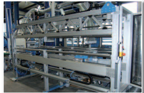
Slitting RB 2 with four sawing stations
