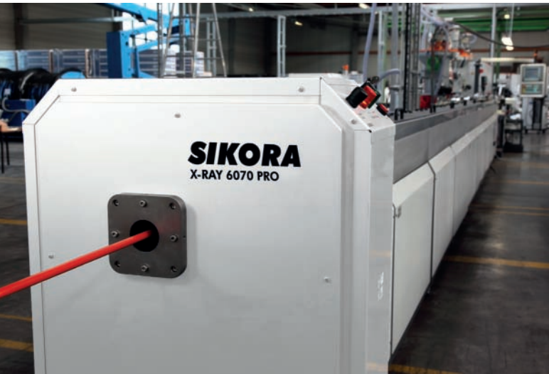
图 4：安装于管材挤出生产线上的X射线测量系统 Image 4: X-ray measuring system installed in a hose extrusion line
